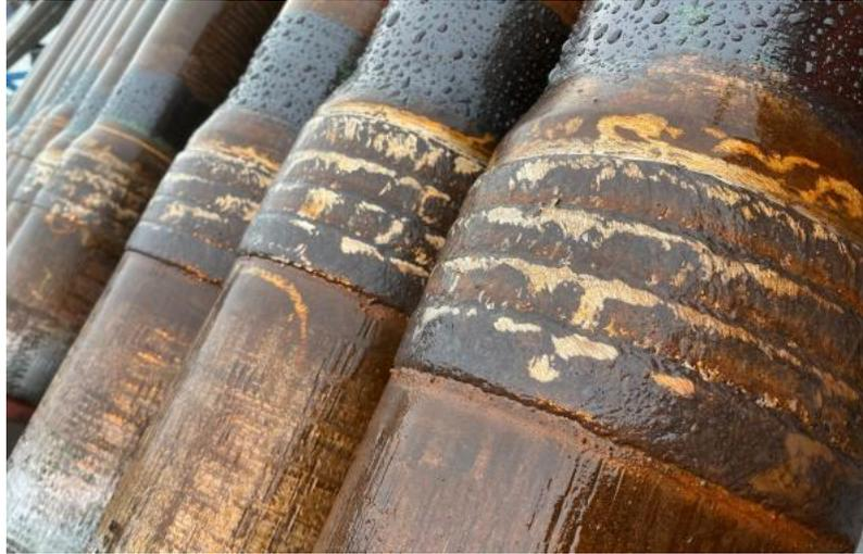
*Figura 17. Hardbanding. (Hardbanding | Castolin Eutectic, 2022)*
