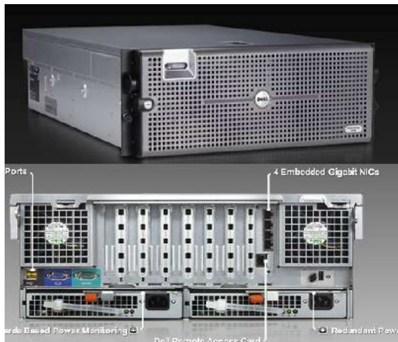
Figura 15 Servidor DELL PowerEdge R900
