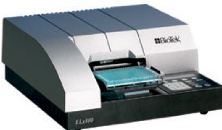
Figura 5. Biotek Elx 800 universal microplate reader.
