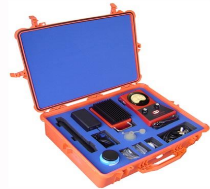
Figura 12. Direct Current Voltage Gradient “DCVG” (Imagen tomada de http://www.cathodicprotection.com/pidcvg.htm )
