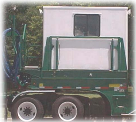
Figura 29. Cabina de control de Coiled Tubing
