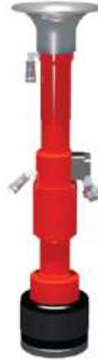
Figura 67 - Pack off, tomado de manual de Lee Specialties.
