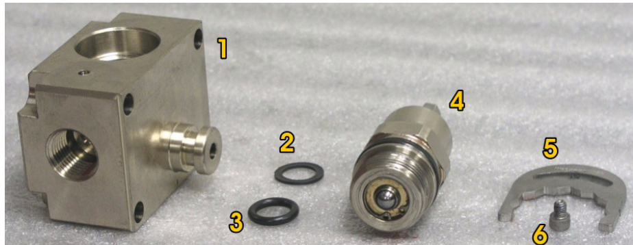
Figure 5-4: Bleed-Off Valve Components
