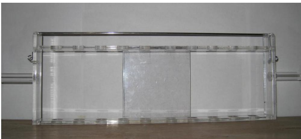
**Figure 1:** Specially designed rack used for phase behavior studies
