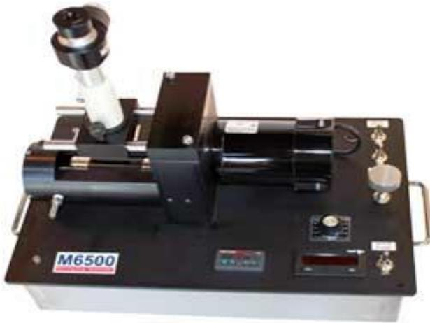
**Figure 2:** Picture showing the M6500 spinning drop tensiometer used<sup>15</sup>
