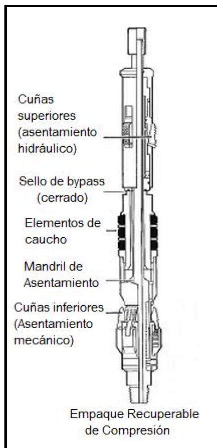
Figura 12 Empaque Recuperable Fuente: Well control for workover operations, Schlumberger
