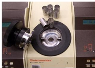
Volume of sample measured using a low pressure pycnometer.
