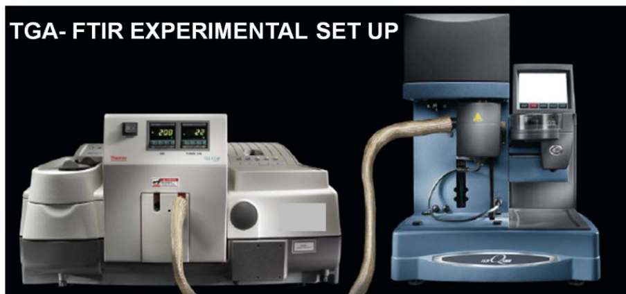
Figura 11. FTIR-TGA Coupling Set up, Montaje Experimental.
