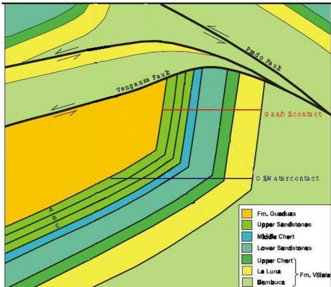
Figura 3. Modelo estructural. Tomado Del paper SPE 71636 Three-Dimensional Modeling of Structurally Complex Reservoirs: The Revancha Field Case
