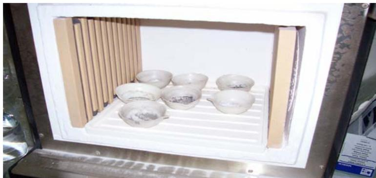
**FOTO 9. MONTAJE PARA DETERMINAR GRASAS EN LAS MUESTRAS
